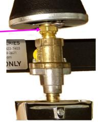
4. An efficient flame is mostly blue with a slight orange tip. Once the flame is large enough, stop loosening and use the silver disk on the air mixer to adjust. Do this on all 3 control valves. Then you're ready to use!
